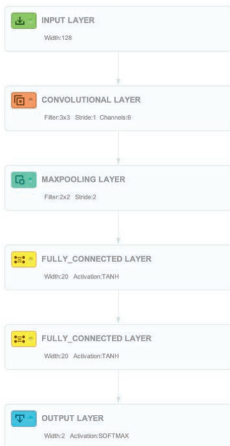
Image 2: Architecture visualized using DeepNetts Platform
